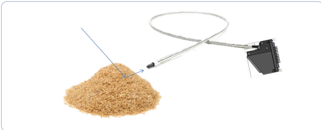
Figure 24: Illustration of coupling into the spectrometer using fiber optics.
