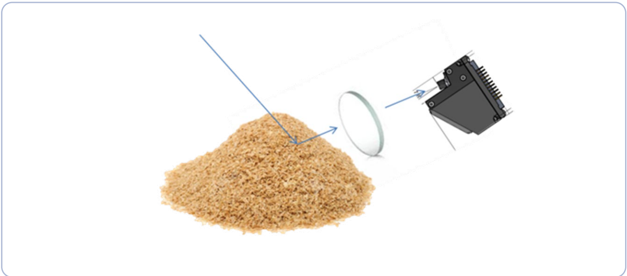
Figure 27: Illustration of coupling into the spectrometer using free space optics.
