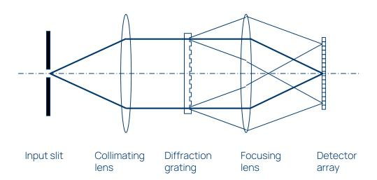
On the following pages are shown two common spectrometer geometries; the transmission grating based and the crossed Czerny-Turner. Also, the figures defines the key design parameters of a spectrometer.
