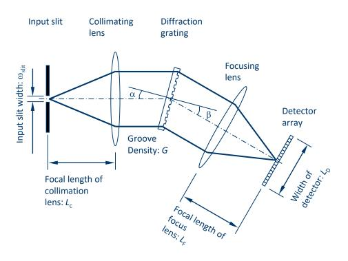
$\begin{array}{ll} \mbox{Minimum wavelength:} & \lambda_1 \\ \mbox{Maximum wavelength:} & \lambda_2 \\ \mbox{Wavelength range:} & \lambda_2 - \lambda_1 \\ \mbox{Resolution:} & \Delta \lambda \end{array}$
