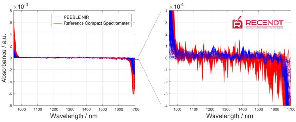
Figure 2: 100% Lines of the PEEBLE NIR compared to the reference compact spectrometer with similar specifications.
