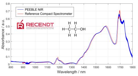
Figure 3: Absorption of ethanol measured in a quartz-glass cuvette with 1 mm path length.
