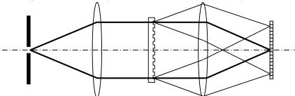
Input slit Collimating Diffraction Focusing Detector grating lens lens array
