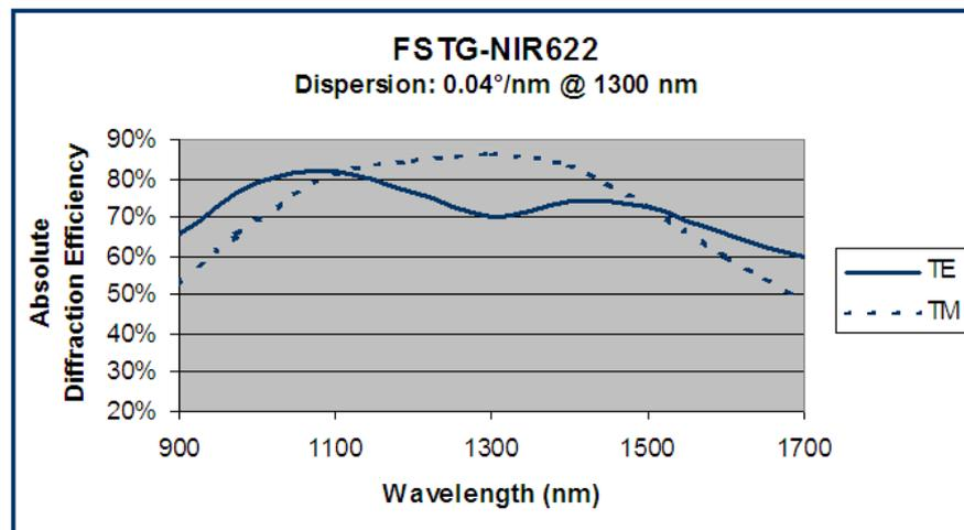
**Figure 3:** Typical diffraction efficiency of Ibsen transmission grating.
