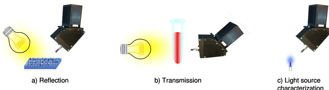
**Figure 1:** Using the ROCK NIR in typical spectroscopic applications.
