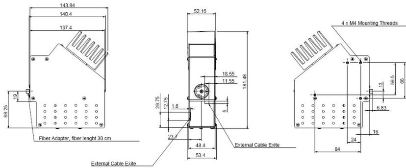
Figure 5: Package dimensions of ROCK NIR
